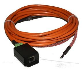
The AKCP ropeFuel sensor is a rope-type leak detector that connects to any AKCP sensorProbe or securityProbe RJ-45 Intelligent Sensor Ports and facilitates the detection of fuel and other liquids.
